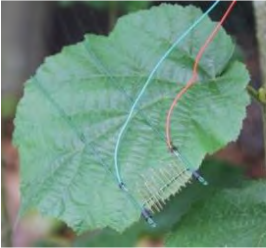
Type \Delta LA-B: Broad leaf version of the \Delta LA-Sensor ( \Delta T Leaf-to-Air)
